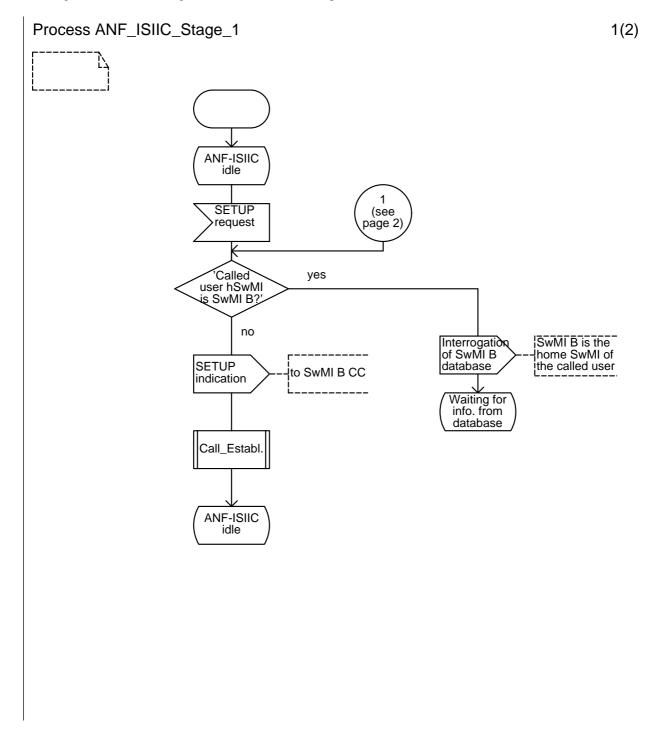
Figure 2 (sheet 1 of 5): ANF-ISIIC, overall SDL Main diagram
