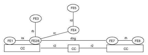
Figure 8: Example relationship between models for ANF-ISIIC and basic call in the case of re-routeing
