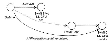
Figure C.3: Interaction with SS-CFU re-routing Forwarded-to user with home SwMI different from SwMI B, having migrated ANF operation by full re-routeing
