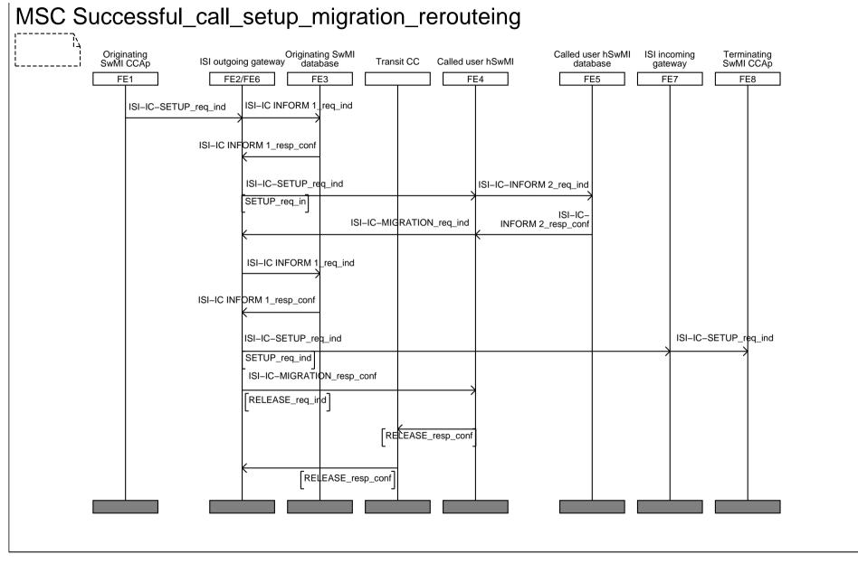
Figure 12: Information flow sequence - call set-up to a called user having migrated from SwMI B, using re-routeing
